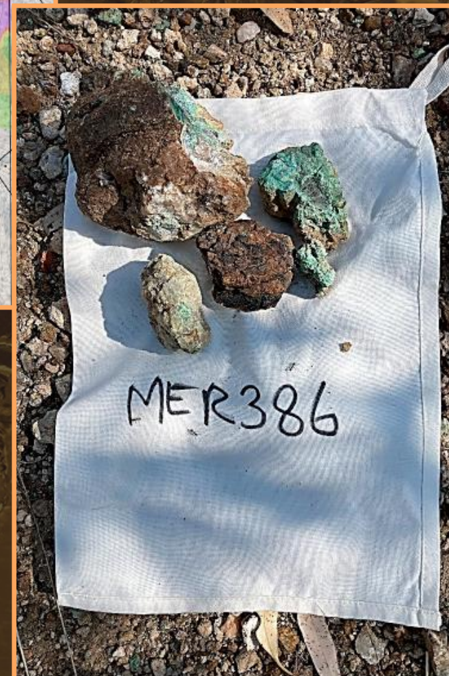
Plate 1: Rock chip (MER386) with 52.8g/t Au and 12.35% Cu
