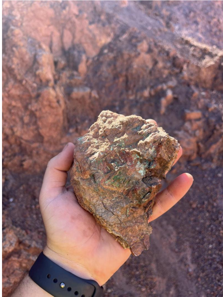
Figure 6: Copper carbonate material grab-sample (MTS_GS004) from the face of the Mt Storm historical open pit, visually estimated grade ~2-4% Cu (assay results pending)
