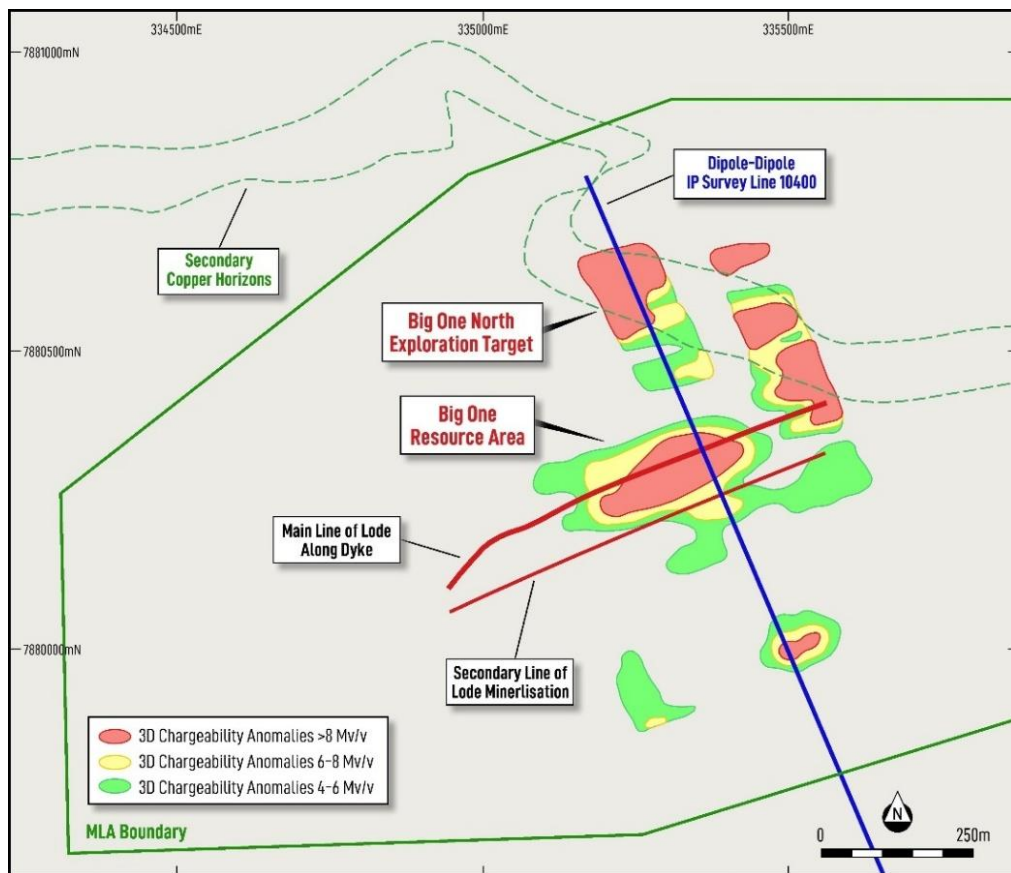
Figure 4: Big One North Exploration Target location plan showing dipole-dipole IP survey Line 10400 over the Big One Resource Area, the Big One North Exploration Target and surrounding chargeability anomalies
