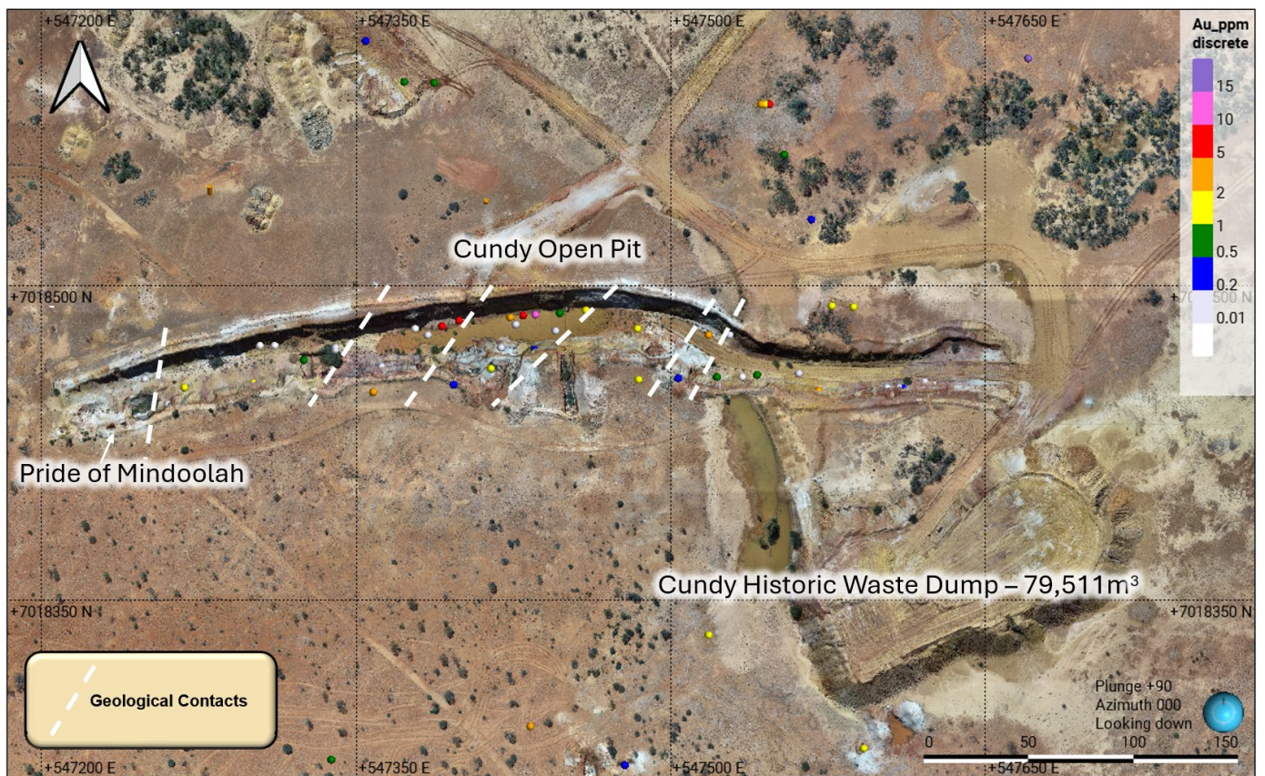
Figure 6. Lidar imagery over of Cundy historic pit and historic waste dump with historic grab samples in plan view (Appendix A – Table 2).
