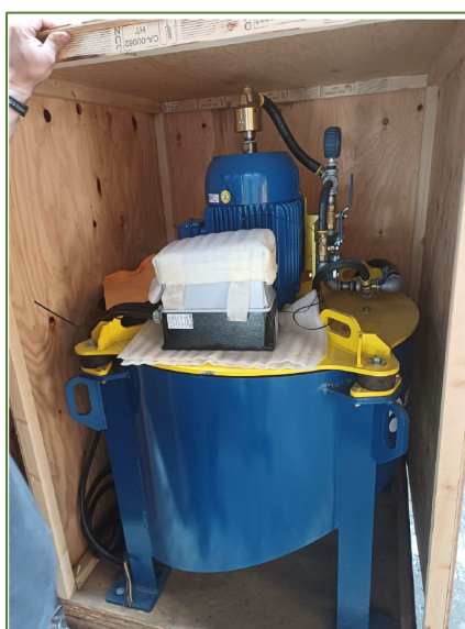
Figure 2 –Preparation of Falcon gravity concentrator for shipment
