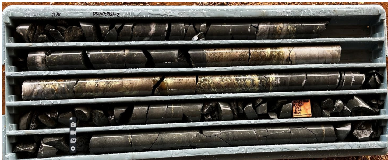
Figure 4: DD26KP1242 ~1m intersection of Hillsborough main lode, comprising of the quartz sulphide vein and massive sulphide. The sulphide mineralisation is a observed was chalcopyrite (20%), pyrrhotite (20%) and pyrite (10%).
