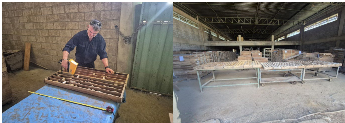
Photo 1: Oceana’s Gareth Reynolds taking pXRF readings of historic core; Photo 2: ~8000m of palletised core available for re-assay.
