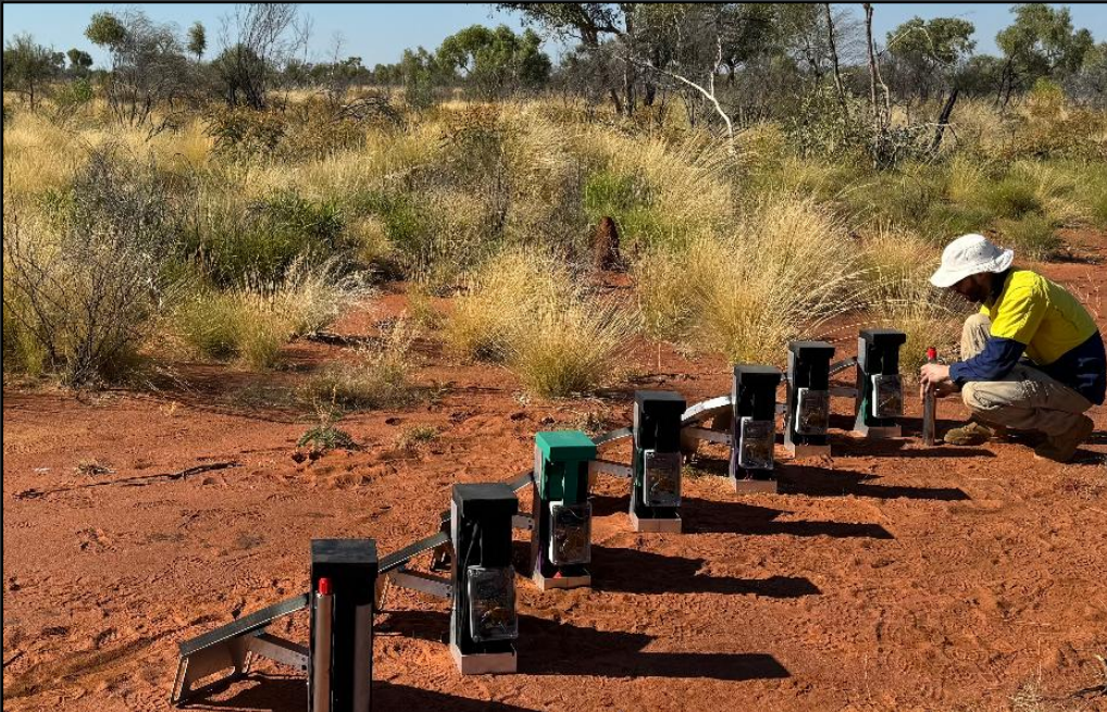
Ambient Noise Tomography sensors being prepared for deployment in the field. The seven sensors shown would each be spaced approximately 250m apart making a total line (array) of 1.5kms for the survey.
