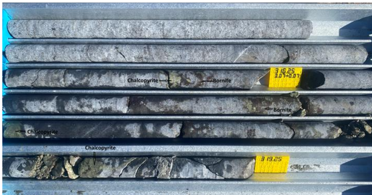
Figure 1: OFMED157 drill core from 313.75m to 319.25m (refer to full reporting in Table 2). Chalcopyrite and bornite sulphide mineralisation is observed from a drill depth of 311.26m to 319.25m.
