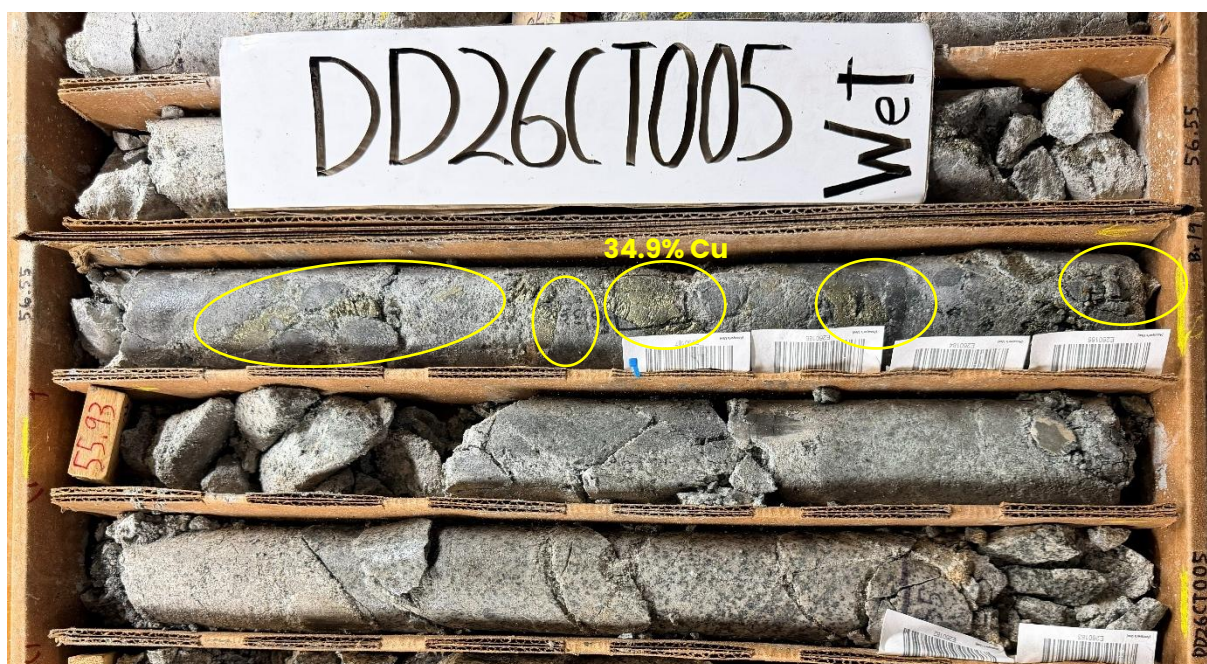
Figure 1: Visible chalcopyrite copper mineralisation between 56–57m down hole DD26CT005 with a spot pXRF copper assay.
