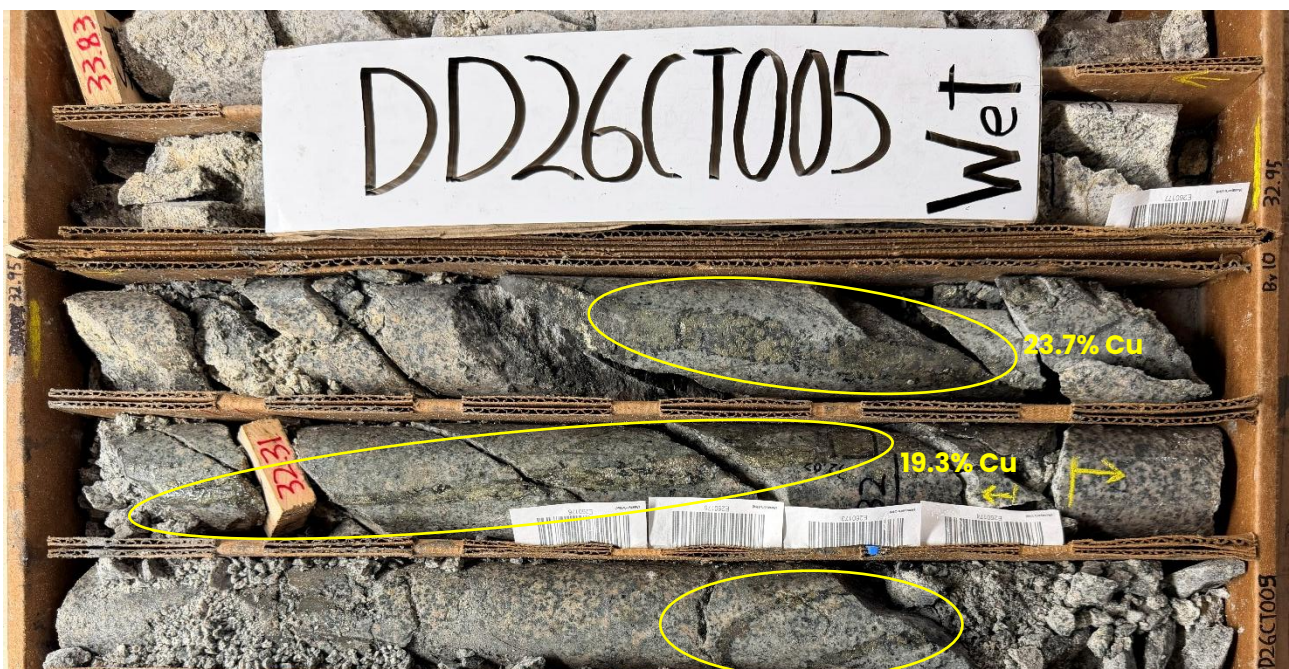
Figure 2: Chalcopyrite copper mineralisation and spot pXRF assays between 31.0-33.0m down hole DD26CT005
