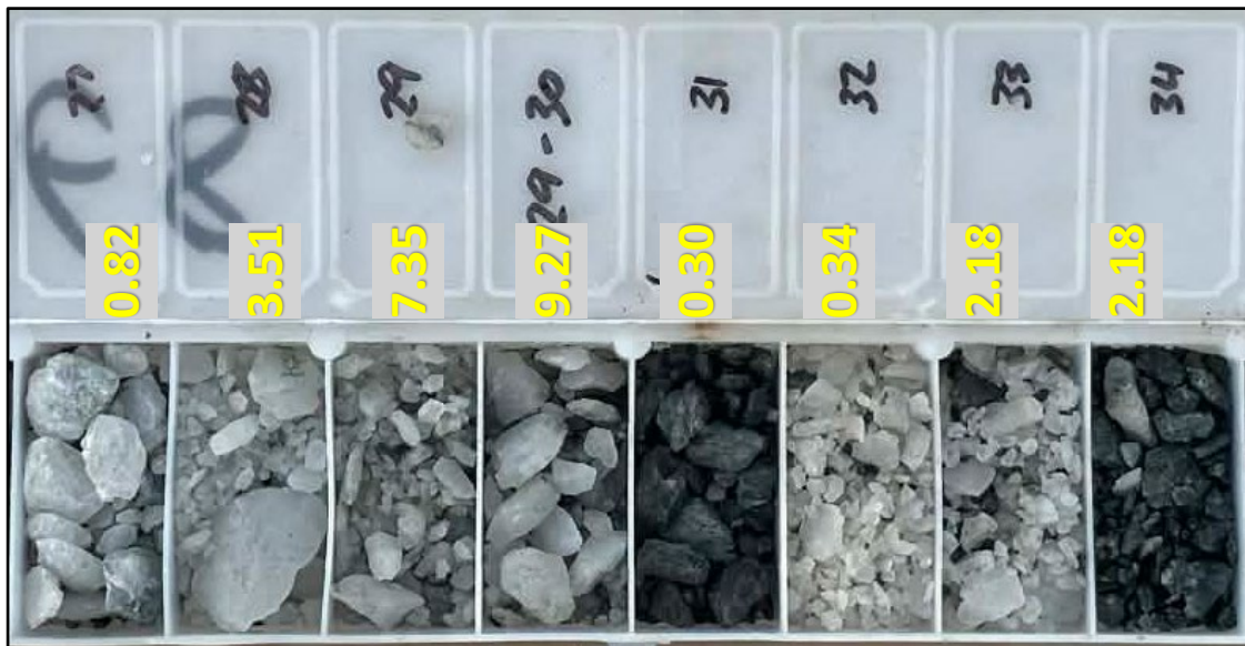
Figure 3. RC chips from 26LSRC068: 27m to 34m, gold grades (g/t Au) shown yellow
