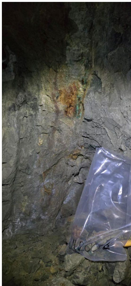
Photo 3. Underground rock chip sample 26MLR00006 from the La Martuca Prospect, showing copper oxide after sulphide associated with structurally controlled quartz-sulphide veining (see Table 1).
