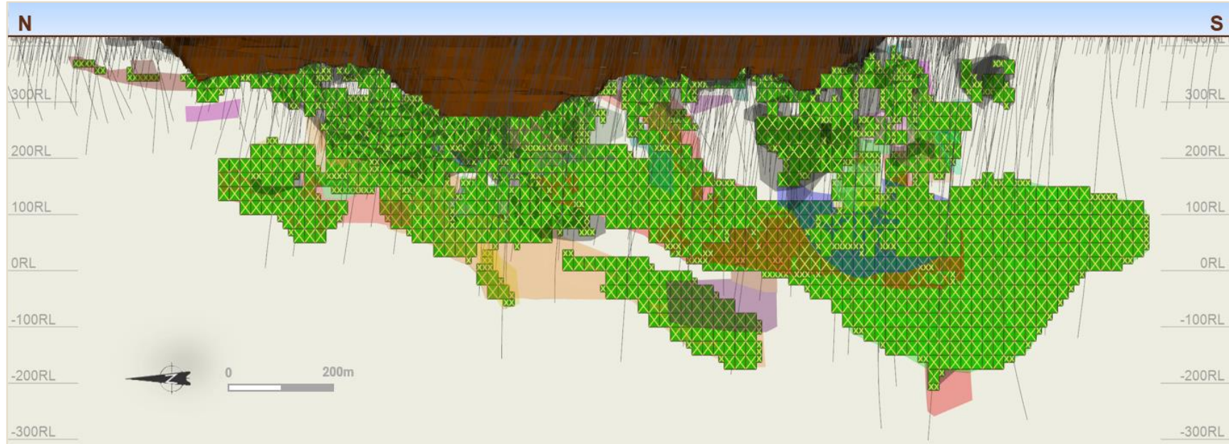
Groundrush long section — green: UG MSO stope wireframes; brown: historical OP shell; ~900 m strike, open down-plunge. Source: TAM ASX announcement.
