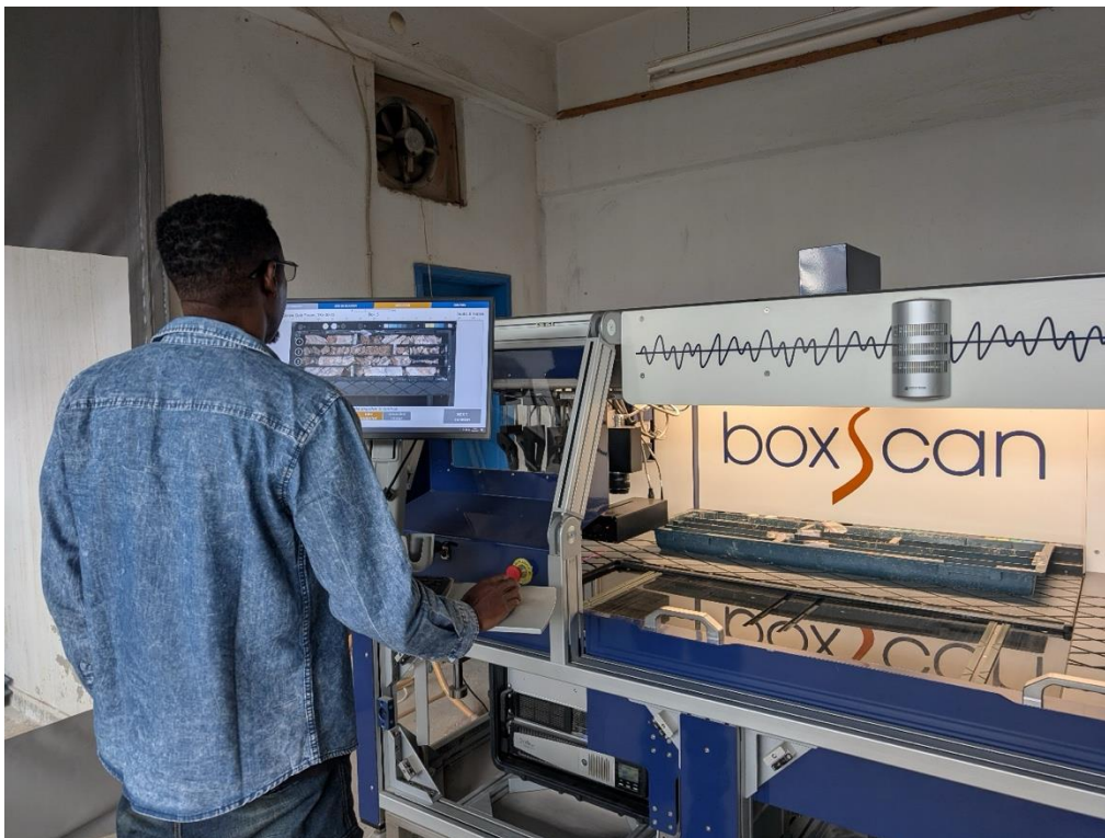
Figure 3: The BoxScan, seen here operating in Türkiye, has been relocated to Dokwe Camp to carry out a range of analyses on the drill core
