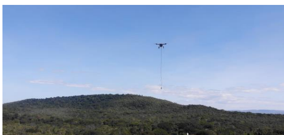
Figure 1. SGB MagDrone in flight over the Palma project area, with the magnetometer suspended on a tether.
