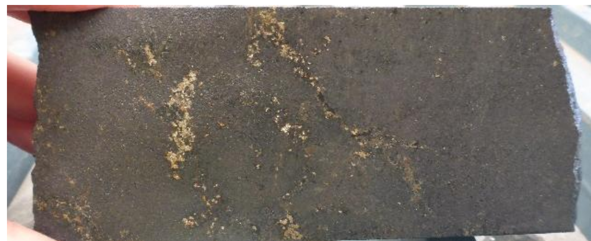
Top: DTD002 - 471m: Hematite alteration with disseminated chalcopyrite + pyrite with cross cutting chalcopyrite + pyrite vein. Bottom: DTD002 - 481.2m: 60cm interval of massive chalcopyrite + pyrite + minor bornite, in quartz magnetite brecciated vein – sample assayed 25.6% copper.
