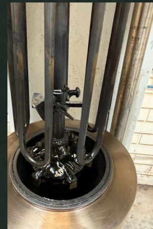
Alpha drill core (top left), Primary pressure leach product (top right), 4L autoclave mixer and process slurry (bottom)
