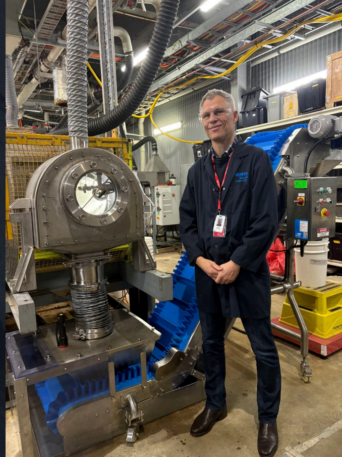
Figure 2: Inspecting the Agglomerator at ANSTO's piloting facility
