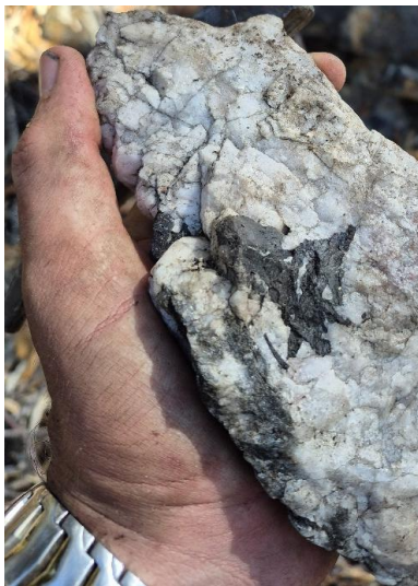
Coarse wolframite crystals hosted by quartz veins at the Lutwyche Prospect, Scamander Project (Samples LW26013 (Left) and LW26006 (Right))
