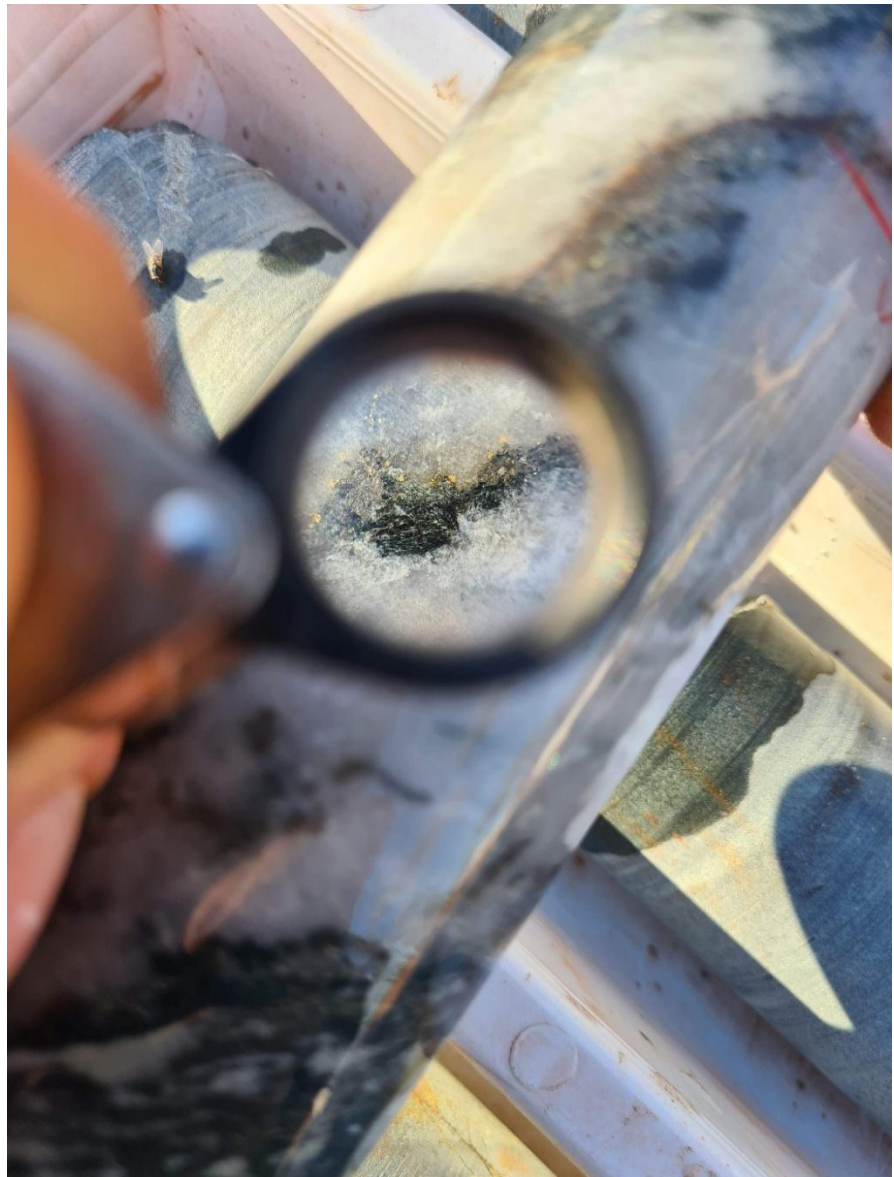
Figure 1: Image of coarse free gold from MZDD001: 76.8-77.0m which assayed 40 g/t Au. Field of view within hand lens ~2.5cm.
