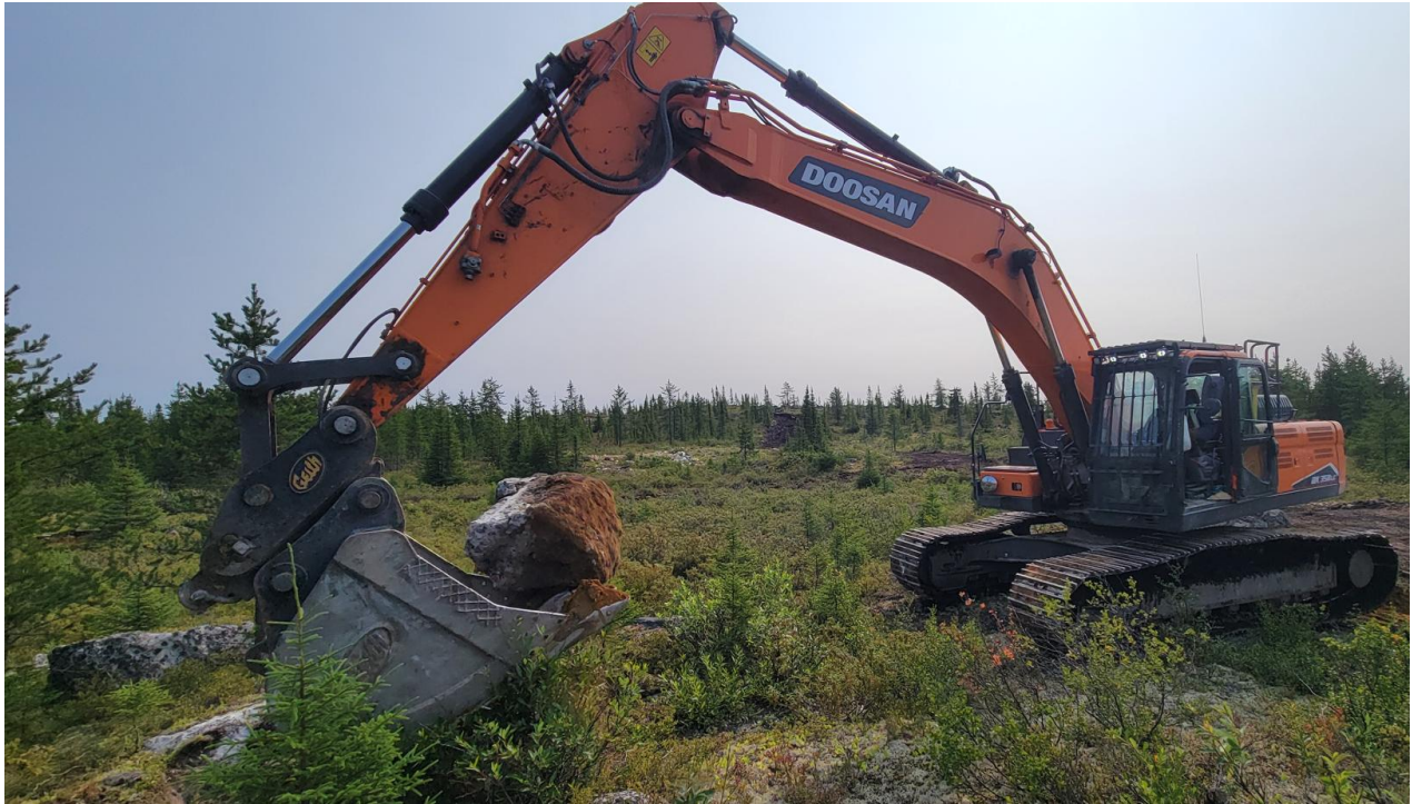
Figure 2: Backhoe collecting spodumene pegmatite mineralized boulders immediately down-ice of the principal CV5 outcrop (adjacent to the southwest side of the CV5 Pegmatite).
