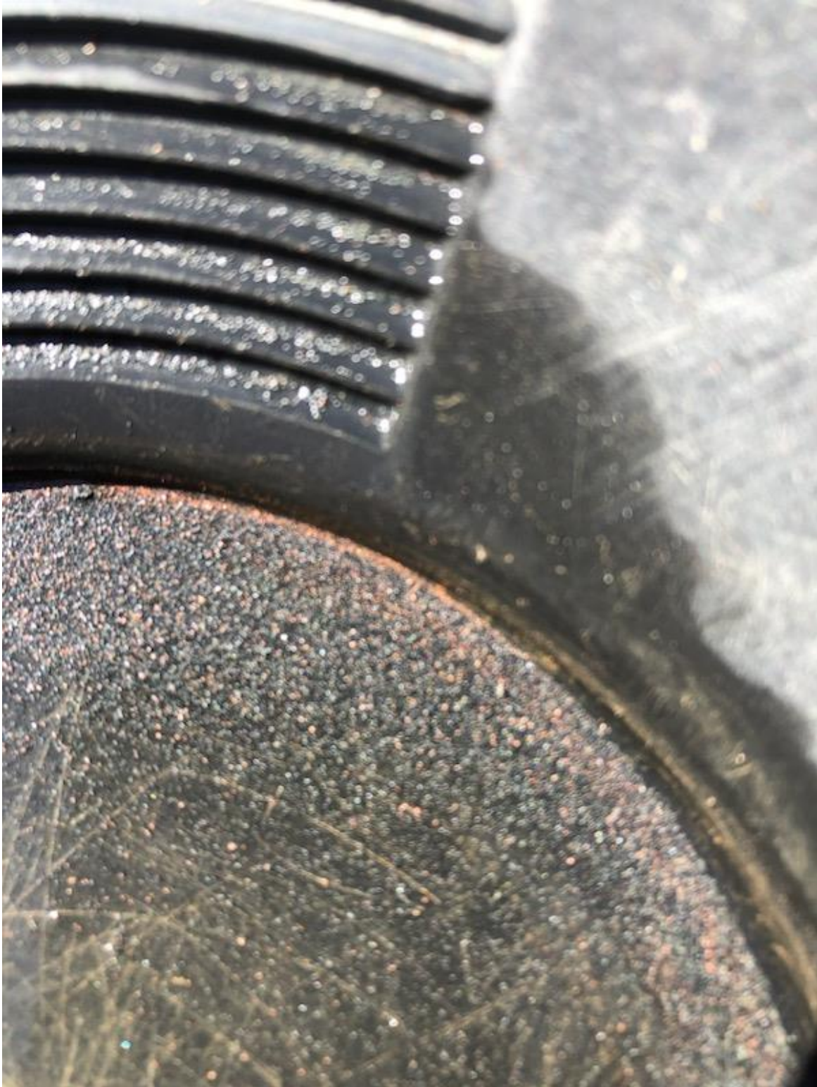
Photo 3. Panned tail showing native copper (pink colour) from drill chips from YRC26-24 (135m to 136m)
