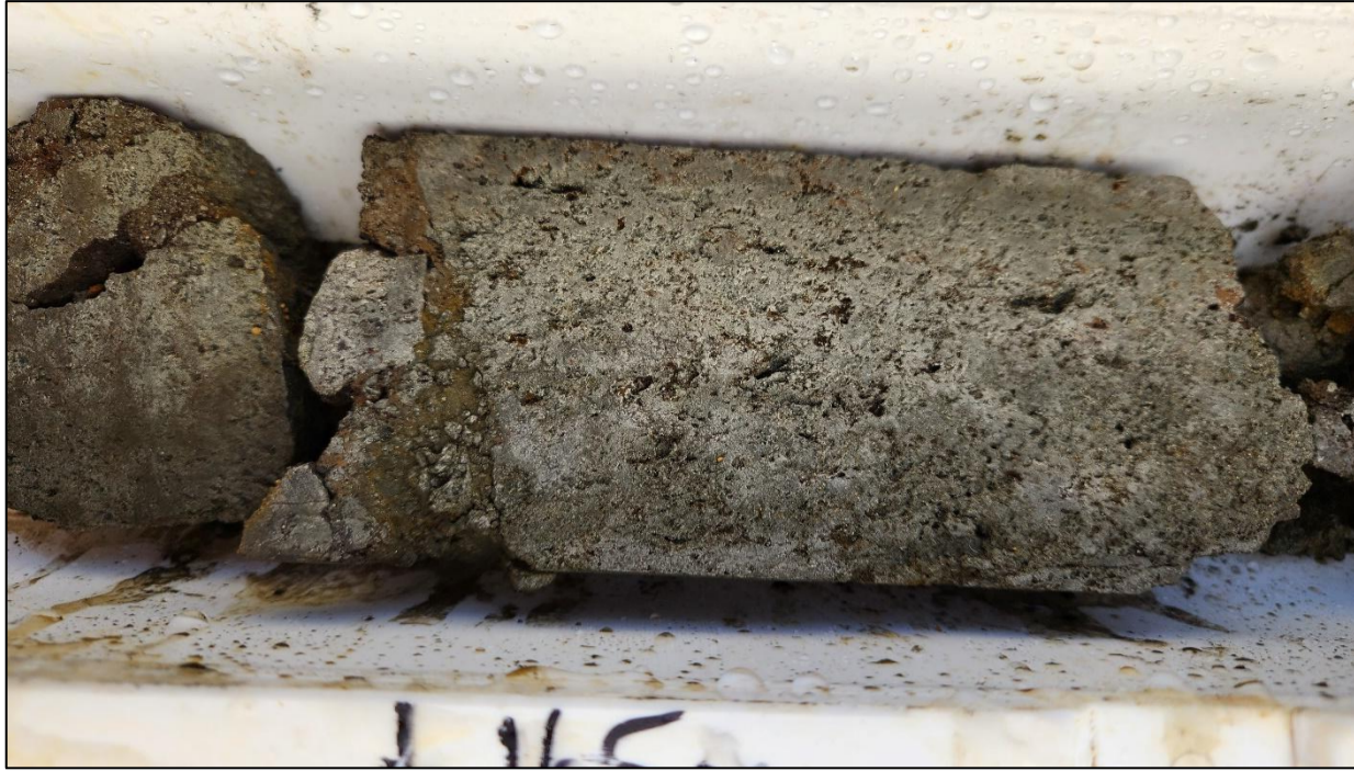
MLJDD018_164.5m_Massive pyrite in Breccia
