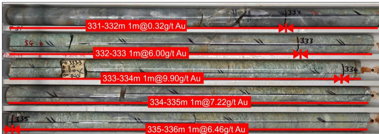
MLJDD042 Silicified ultramafic with fuchsite Alteration
