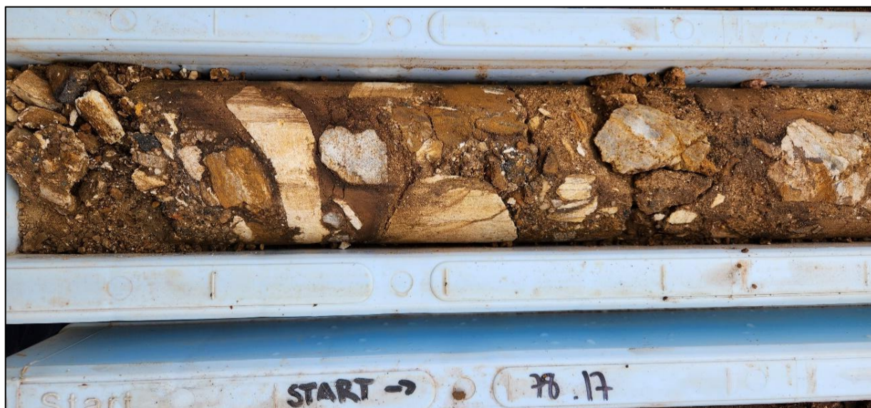
MLJDD020_178.0m_Polymictic Breccia with silica-pyrite clast
