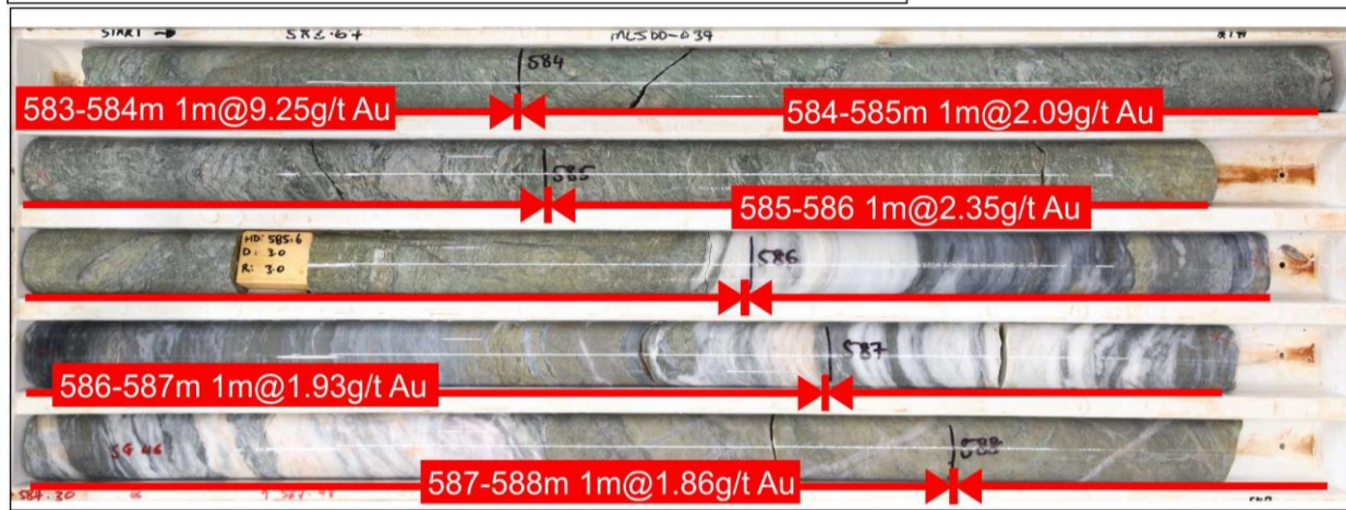
MLJDD039 Silicified ultramafic with fuchsite Alteration
