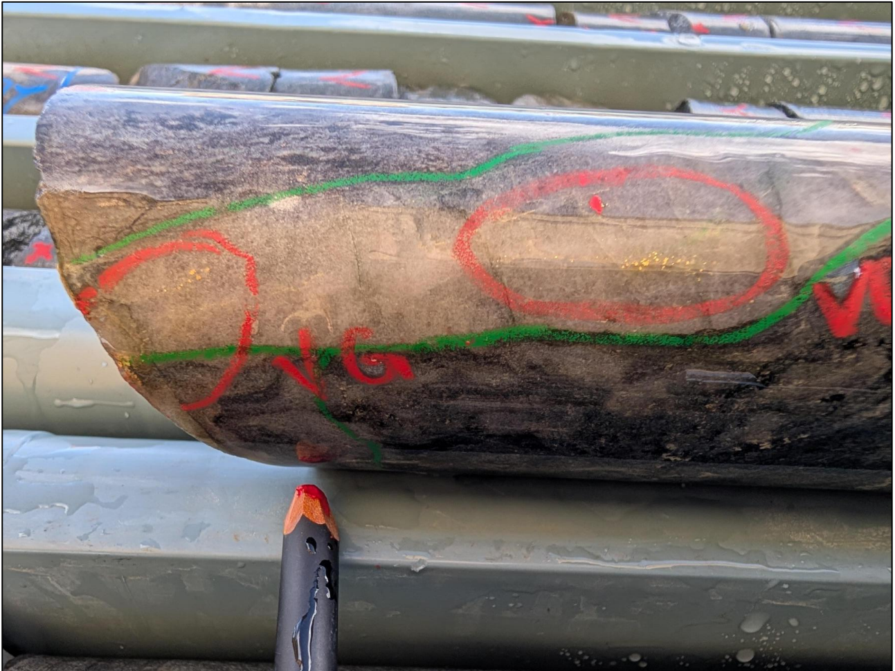
Figure 2 – Gold mineralisation located within a quartz vein hole 26HBBD044. The interval grades 4.20m @ 42.43g/t Au from 289.63m including 1.37m @ 126.93 g/t Au from 290.84m (refer Table 1). Core width is NQ2 and ≈ 50.5mm in diameter for scale
