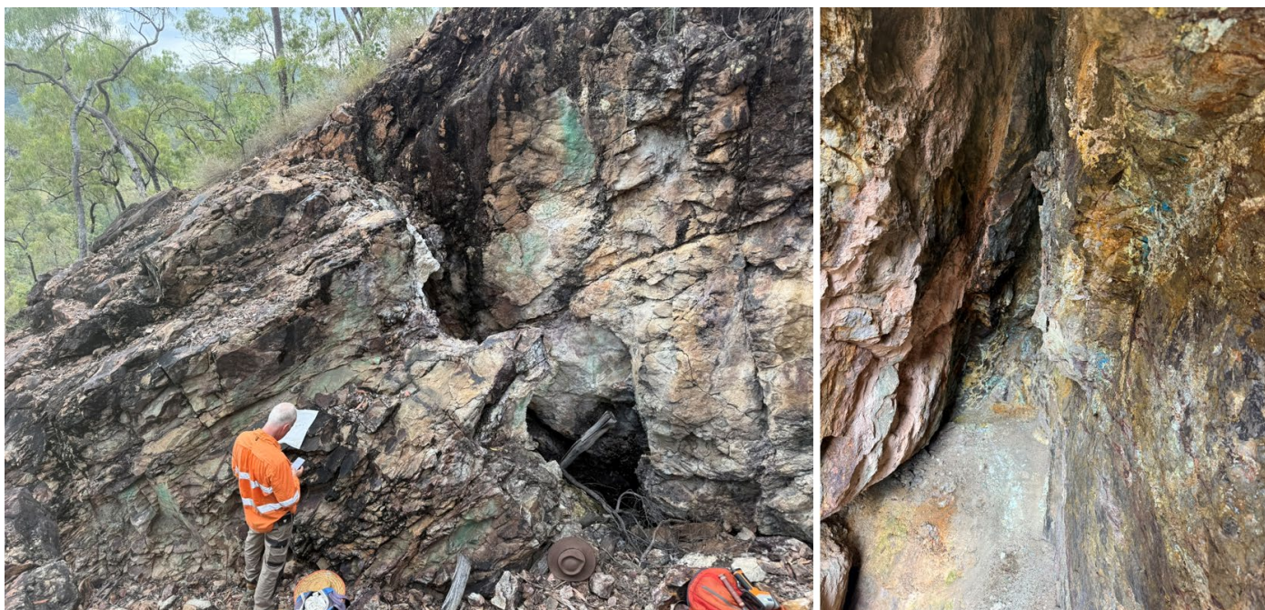
Figure 5 Left: Malachite (copper carbonate) on the entry to an historic mine (the mine adit entry is to the right, out of frame). Right: a gossanous, malachite and azurite coated vein in a mine adit.
