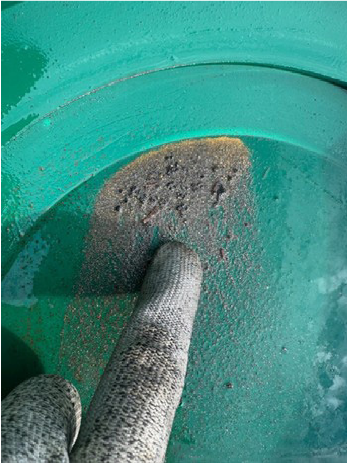
Challenger plant operators use gold panning to observe plant performance.
