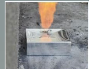
LIB Penetration Test
