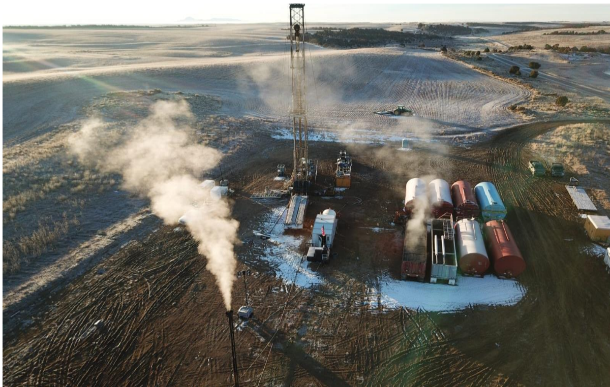
Figure 4: Jesse-1A flow test venting reservoir gases and helium through the flare stack in (Grand Gulf, 2022)
