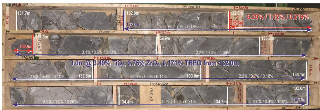
Figure 7 – NWOR-03 core photos with individual grades (white; TiO 2 % / ZrO 2 % / TREO%) and weighted average assay grades (blue: 2.0% TiO 2 cut-off; red: 5.0% TiO 2 cut-off).
