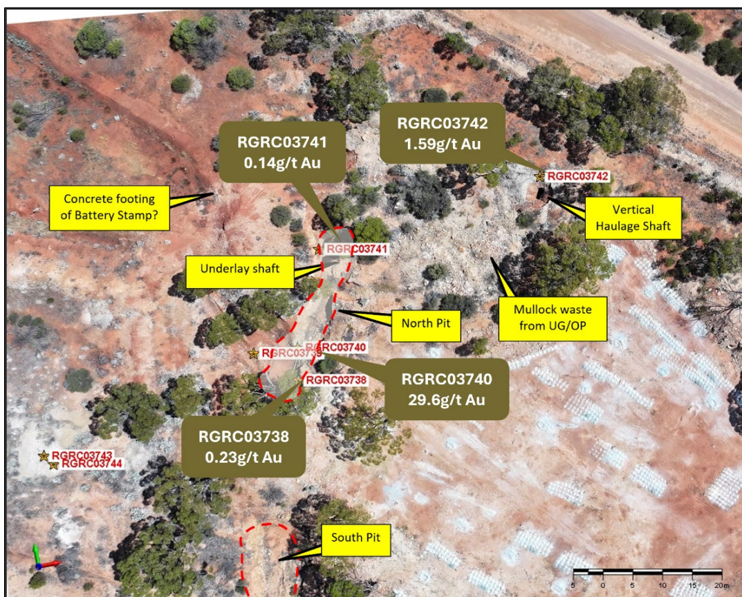
Figure 3: Repeater prospect sampling locations with image showing recently completed drilling
