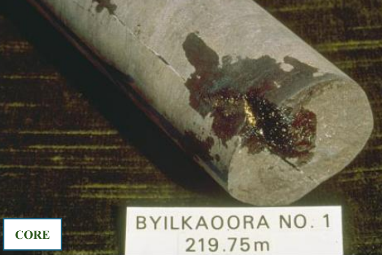
Oil bleeds Observatory Hill Formation Byilkaora 1; core, 219.75 m (Photo 44388)
