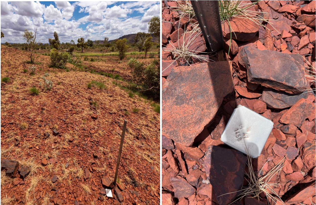
Figure 3/4: Tenement boundary peg for the south eastern point of Mining Tenement M47/1450.
