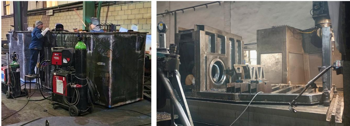
Manufacture of Power Take-Off Modules
