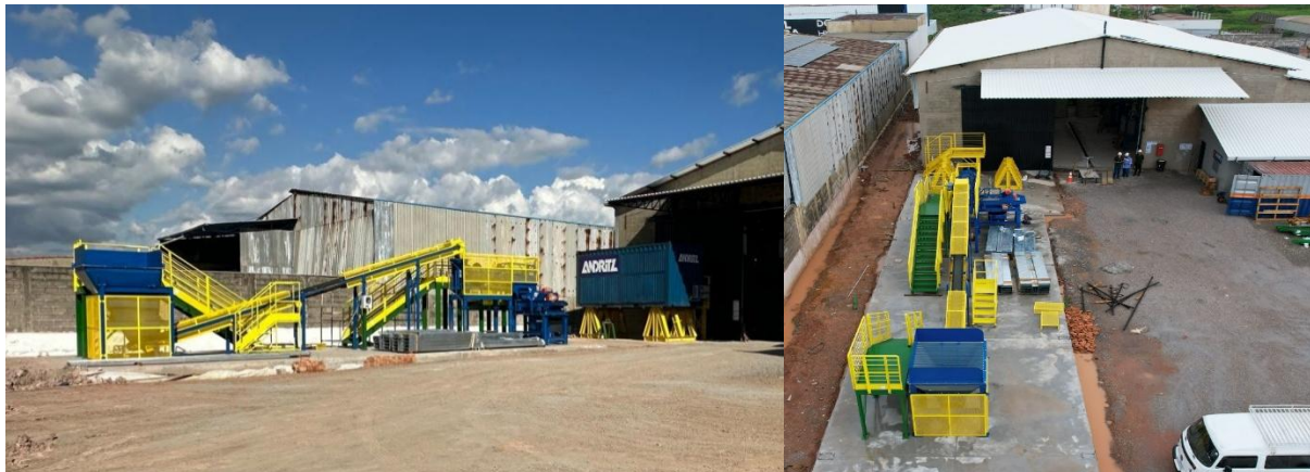
Figure 1: Ore scrubbing and handling package sized for 100kg/hr and Residue Ore Filter Press.
