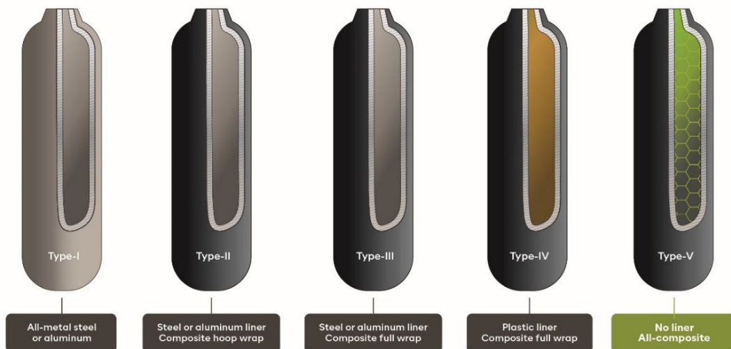
Figure 2: Five common pressure vessel types including the Type-V tank.
