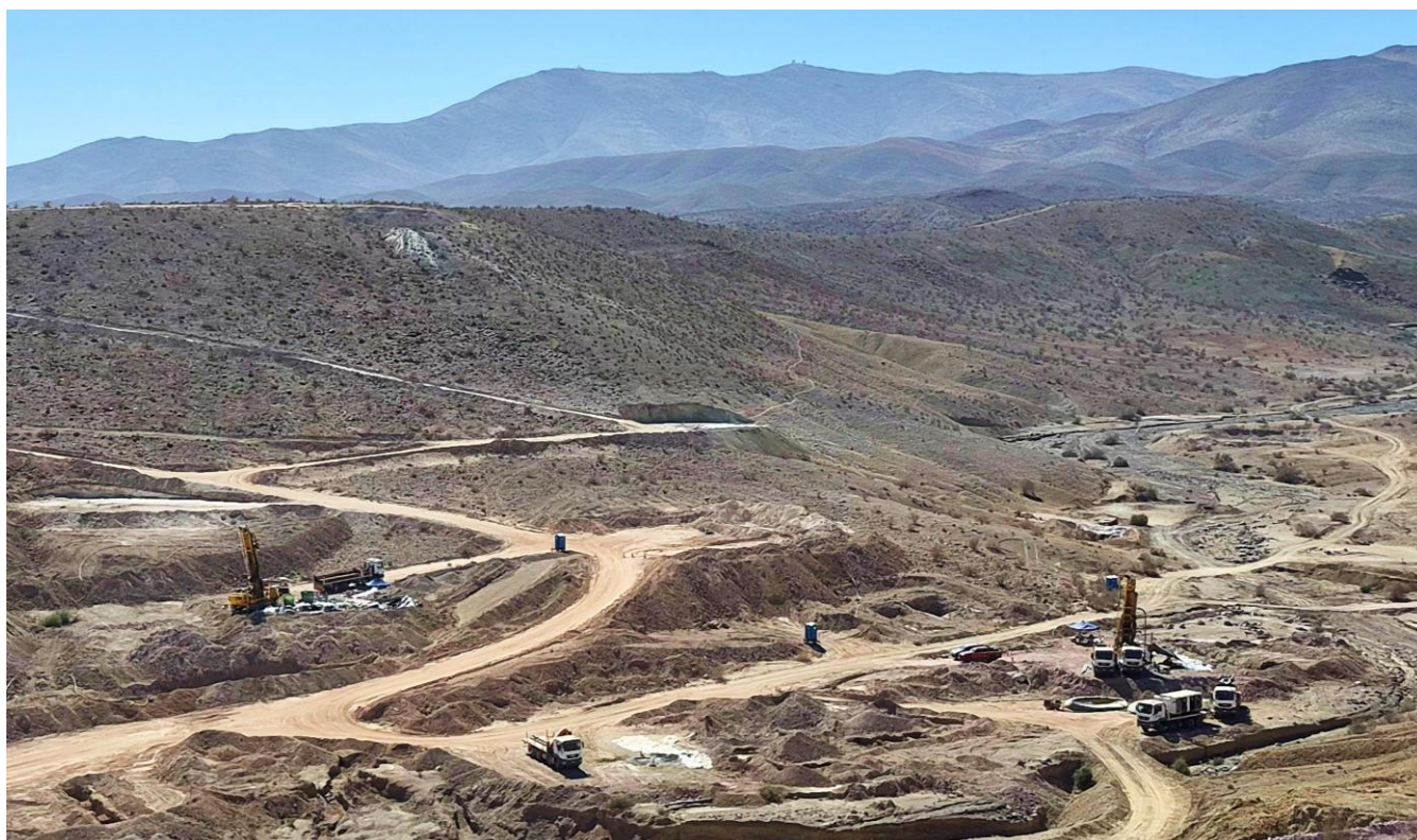
Diamond and RC Drill rigs accelerating development of the La Verde Cu-Au discovery
