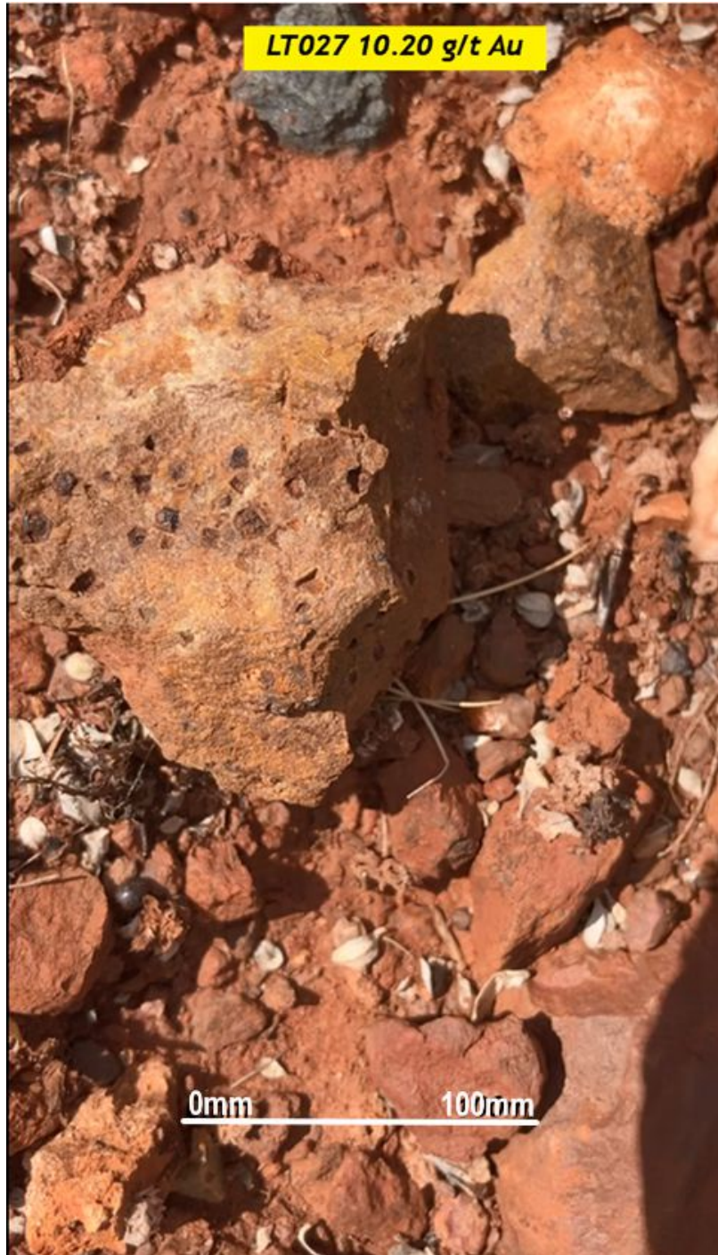
Figure 2 Rock sample LT027 displaying Euhedral sulphide casts providing a gold grade of 10.20 g/t Au
