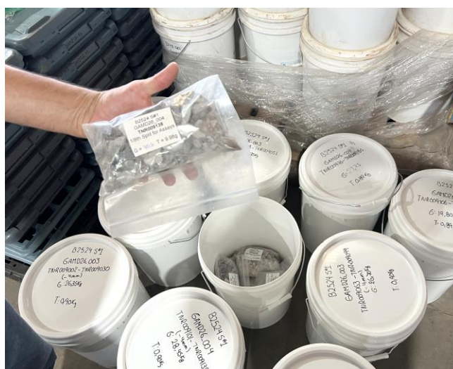
Figure 5: CCP samples on arrival and after crushing at metallurgical laboratory
