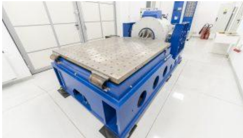
Vibration system (shaker)
