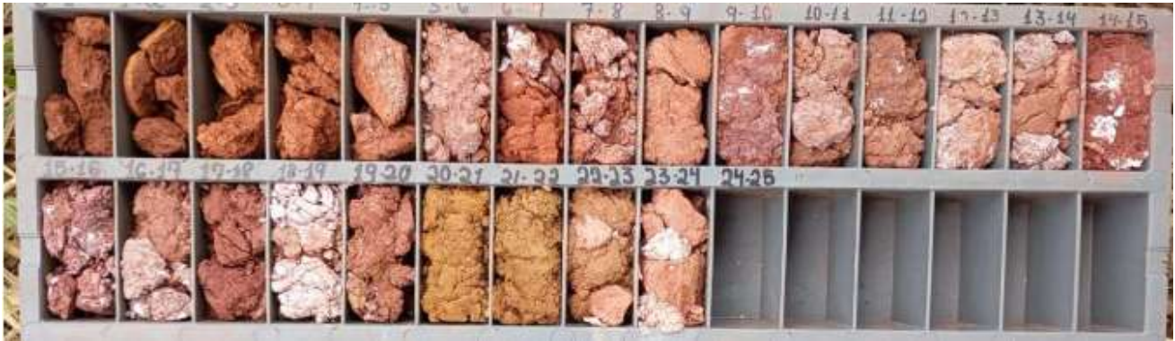
Figure 6: Auger drill cutting chip library from auger hole CDE-AD-007.
