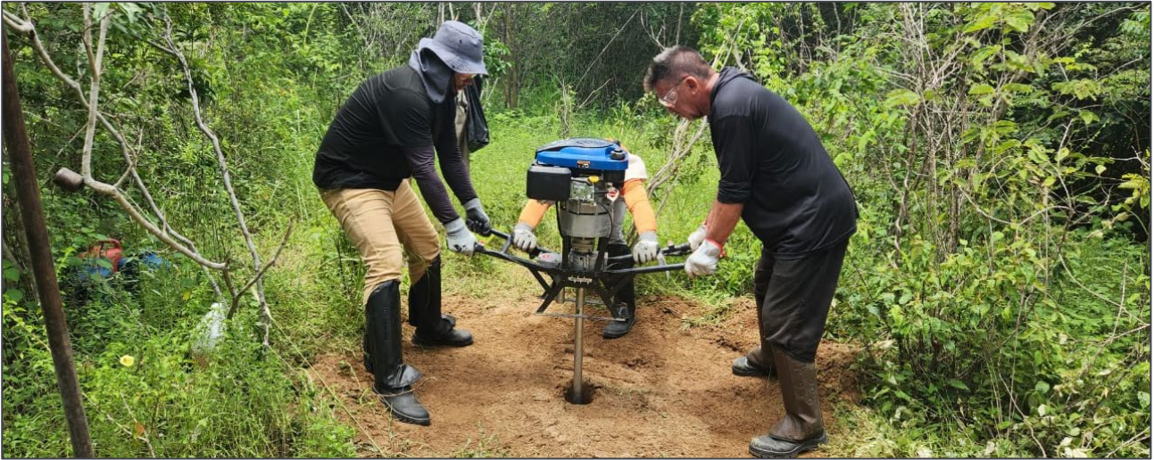
Figure 1: Auger drilling at the Company's Itambe Project location at the southern end of the highly prospective Rocha da Rocha Rare Earth Province.
