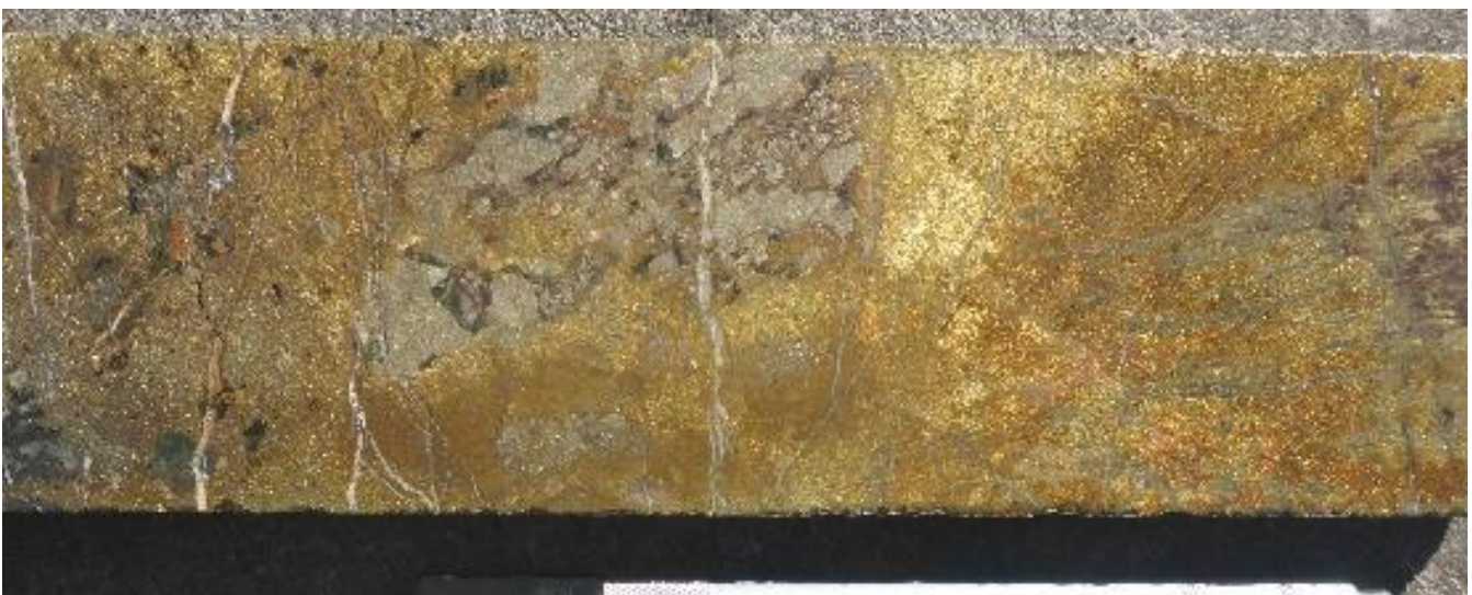
Figure 1: DTD002: 481.2m 60cm interval of massive chalcopyrite + pyrite + minor bornite, in quartz magnetite brecciated vein – sample assayed 25.6% Cu & 1.29g/t Au.
