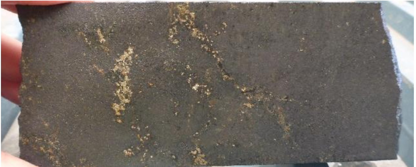
Figure 2: DTD006b: 520.1m Intense magnetite alteration with disseminated pyrite + chalcopyrite – sample assayed 0.30% Cu & 0.16g/t Au.
