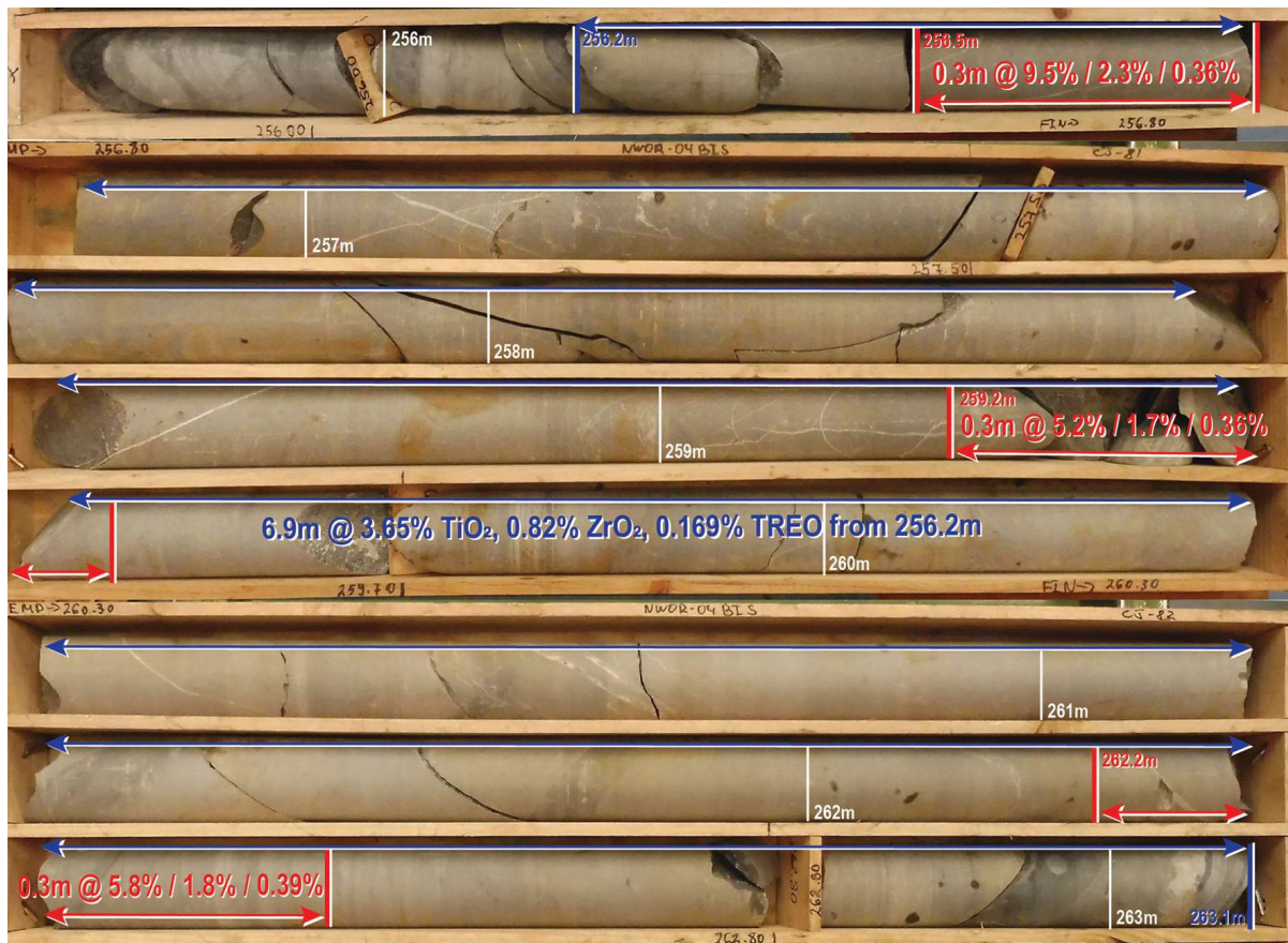
Figure 4 - NWOR-04bis core photos with weighted average grades (blue: 2.0% TiO 2 cut-off; red: 5.0% TiO 2 cut-off).
