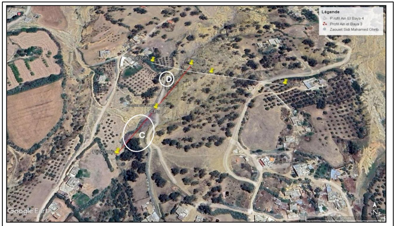
Figure 7. Location Geophysical Sections 3 and 4 on a Google map base (pre-independence open pit mining. C: mine spoils, D: tunnel).
