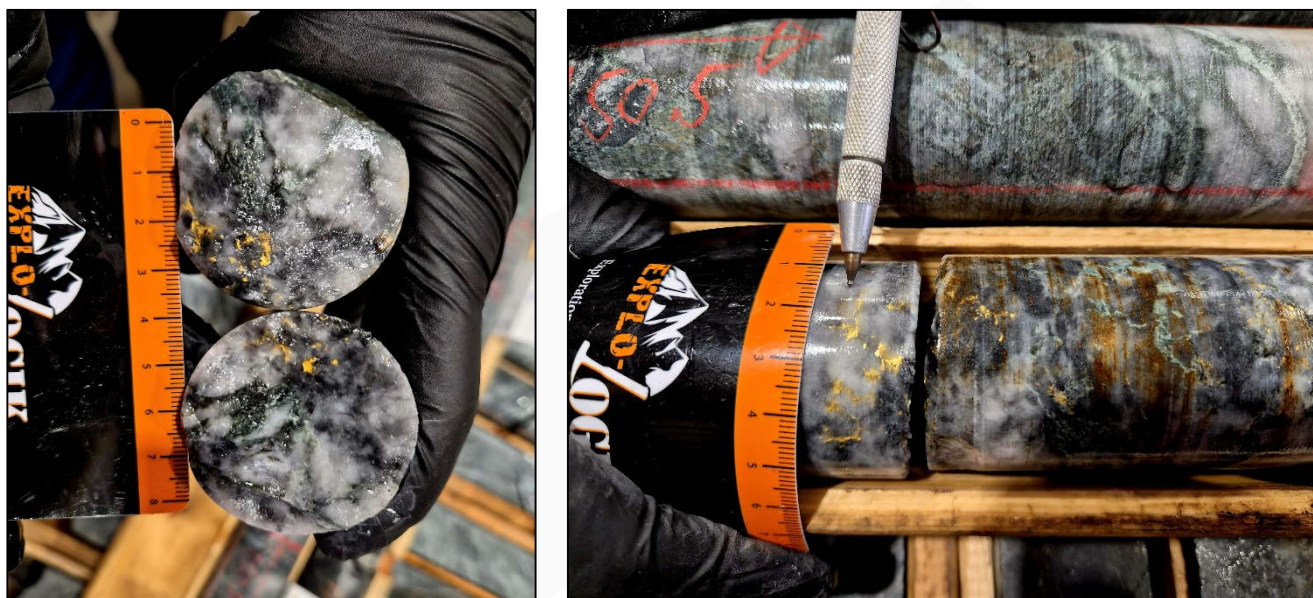
Figures 1 and 2 – Visible gold in quartz veining, drill hole AS-26-793 (~152.05m), Astoria, Rouyn Gold Project
