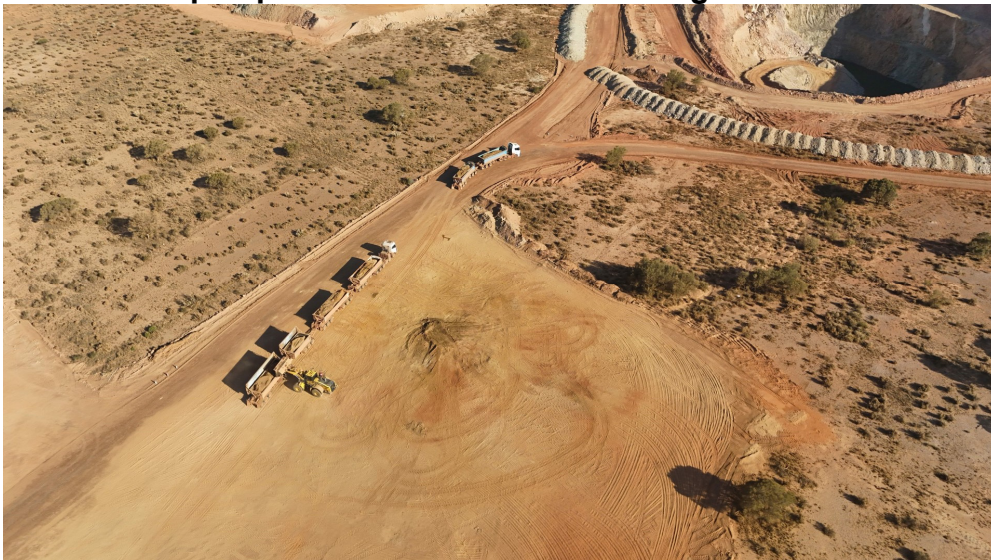
Photo 3: Final ore being loaded onto haulage trucks at the Neta ROM 24 January 2026. Neta open pit and closure bund in background
