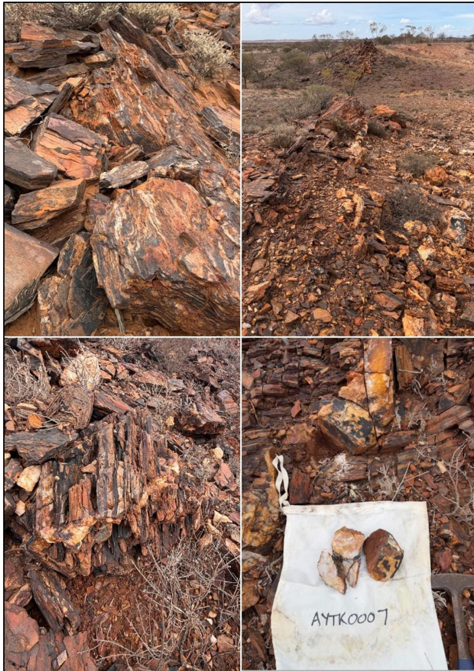
Figure 4: Top Left – Chert-magnetite zone in BIF (Brunswick Hill); Top Right – Quartz veining and shearing along BIF (Mt Sandy); Bottom Left – Extensional quartz veins in BIF (Mt Sandy); Bottom Right – Rock-chip sample AYT0007 of an oxidised (ferruginous) quartz vein containing iron oxides (goethite and limonite) taken from outcropping BIF in the Mt Sandy Area. Visual estimates are based on geological observations, and it is considered no economic mineralisation is present in this photo. Laboratory assay results are required to determine potential grade and potential economic mineralisation, if any.
