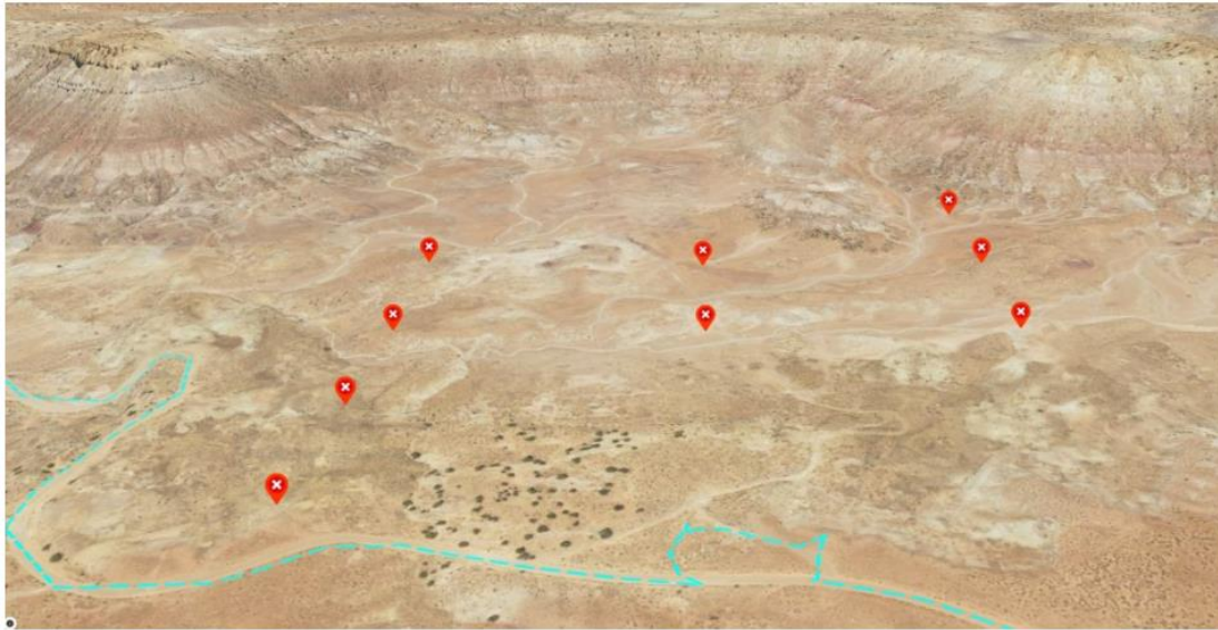
Figure 4: Plan showing the proposed drillhole locations to be carried out east of the “Cactus Rat” mines.
