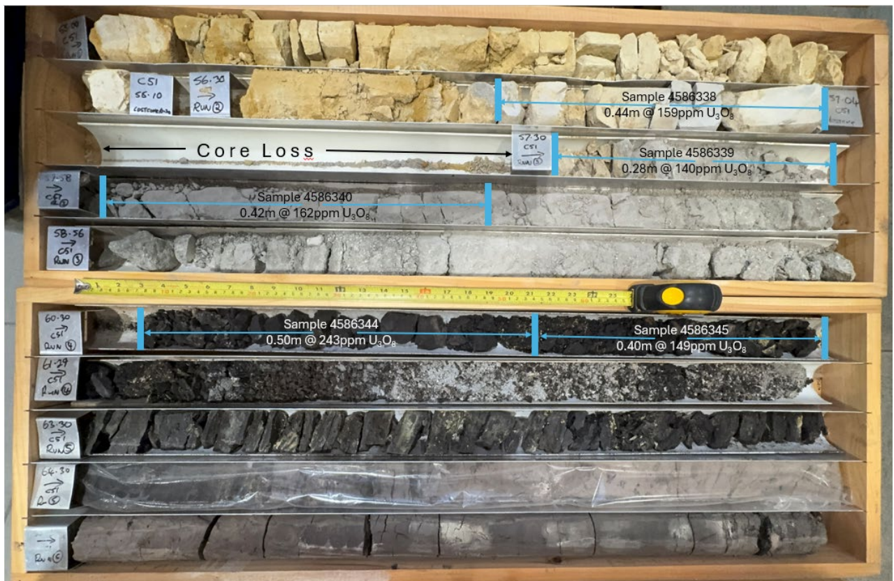
Figure 3: Core hole C51, with significant uranium assay intersections marked. Note redox boundary becoming evident in the sample 4586338 sample interval.
