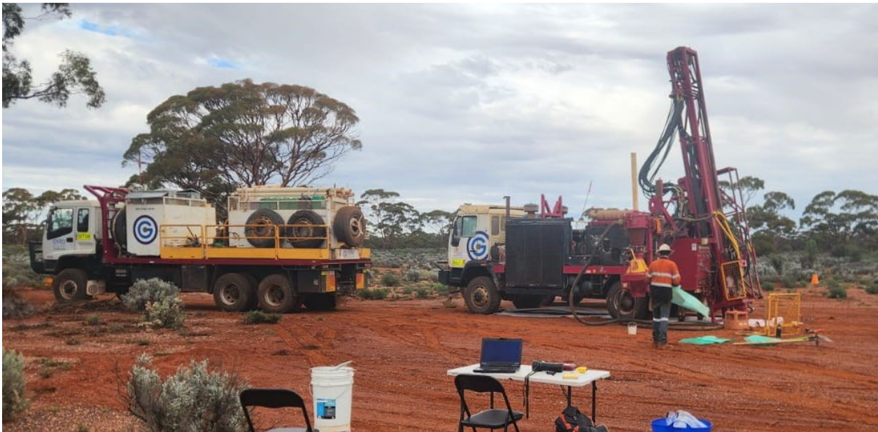
Figure 1. RC Drill Rig on Site at the Kanowna Gold Project
