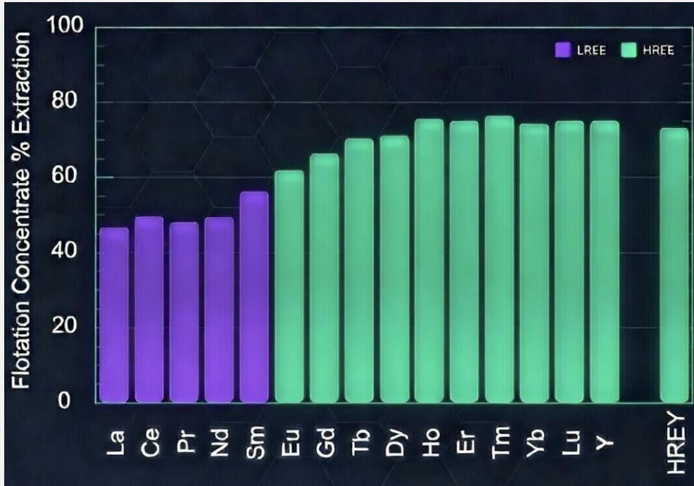
Figure 2. Graph showing the increased extraction of Heavy Rare Earths vs Light Rare Earths.
